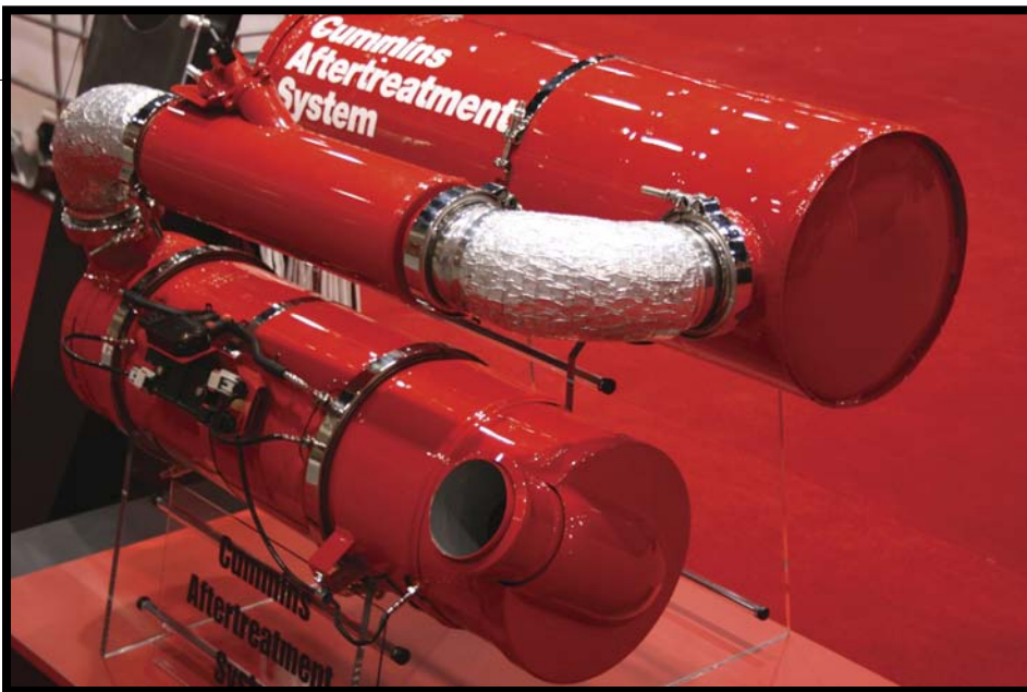
Cummins combined diesel particulate filter and selective catalytic reduction chamber. Both have sensors and controls to make it a complex assembly, which may have its share of maintenance issues.
