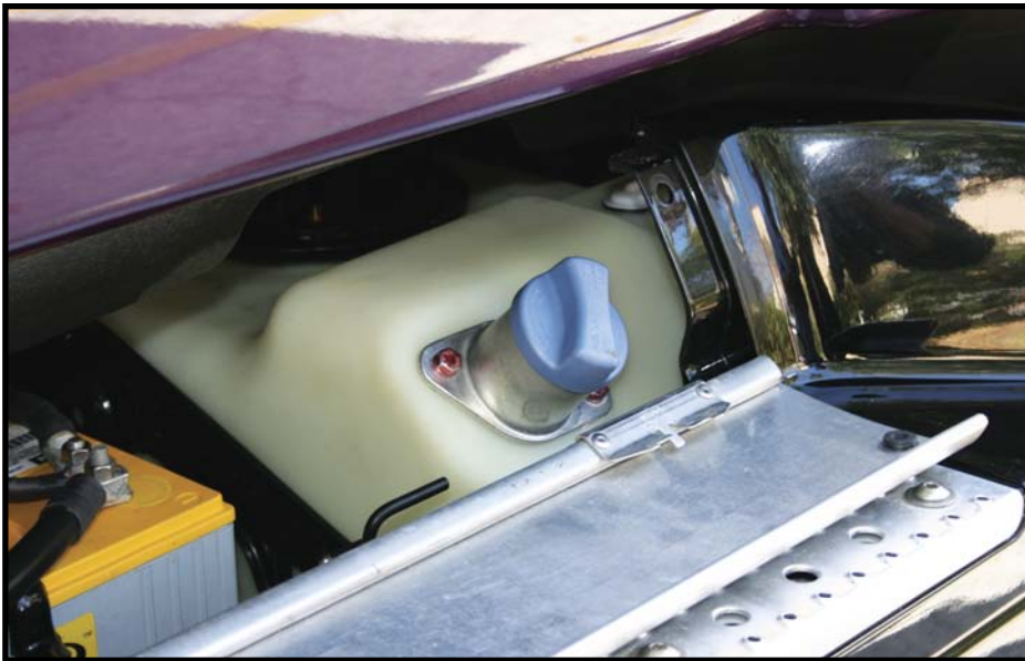
SCR tanks are sized to make filling only half as frequent as the fuel tanks. The filler neck is smaller than a diesel nozzle and coded blue to avoid mixing the fluids when filling.
